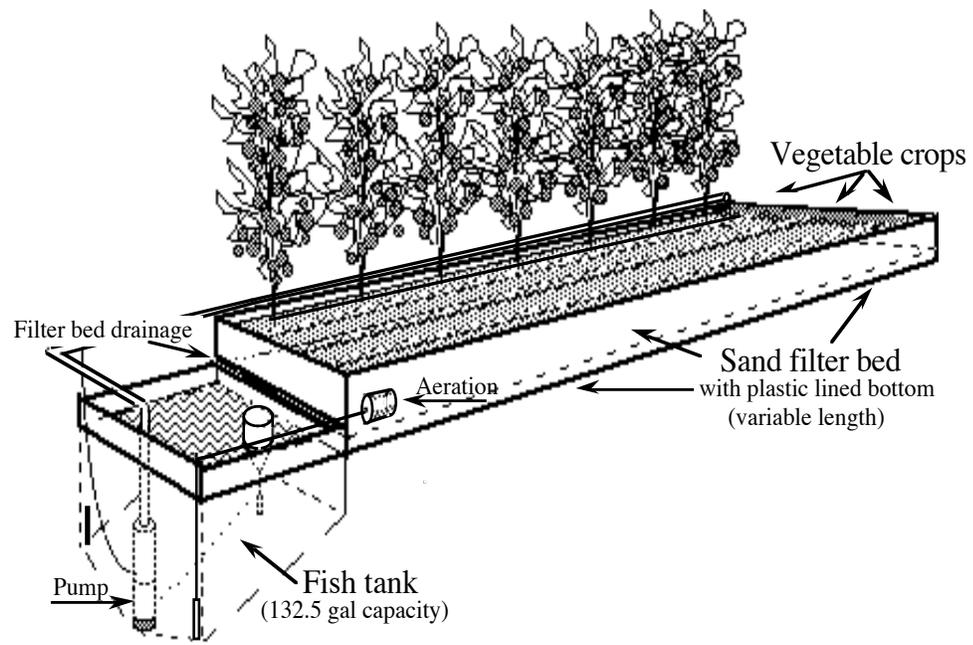
Fig. 1. Schematic diagram of the integrated aquaculture-olericulture system.
